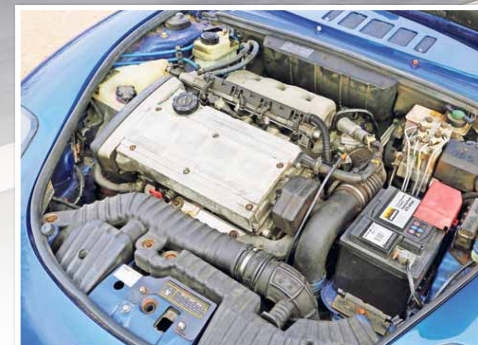
Boisterous and lusty, the 1747cc twin-cam beneath the Barchetta's bonnet is perfect for the job of seducing the driver.
